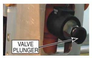
Figure 3-6. Manual Lowering Valve (Jib)
